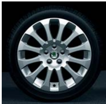
6.5J x 16" Comet alloy wheels for 205/45 R16 tyres.
